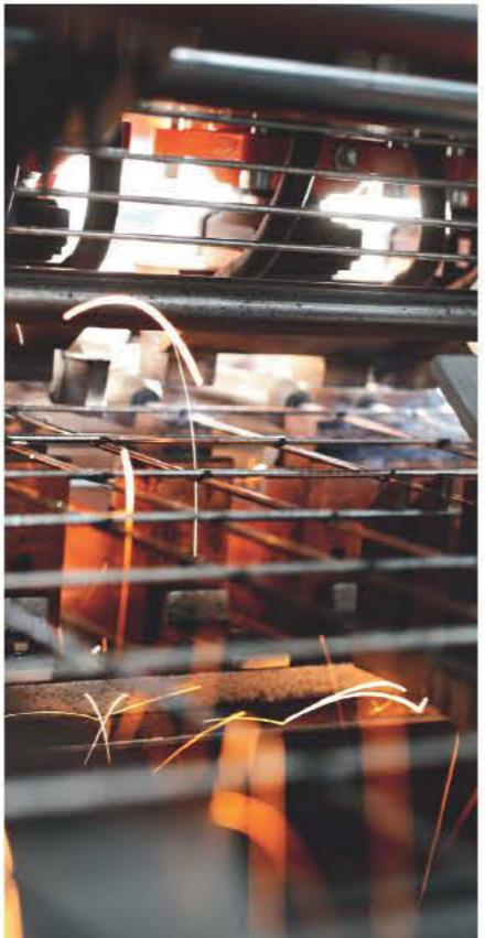
Schnell Home machines produce a panel that consists of a polystyrene sheet assembled together with welded wire mesh.
