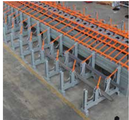
3. RACK: The rack allows collecting the cut bars and making them up into bundles when further processing is not required.
