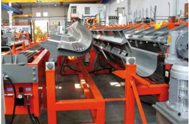
16. Lifting buffer. It receives the bars from the Shearline pockets and lifts them onto the roller track of the bending robot.
