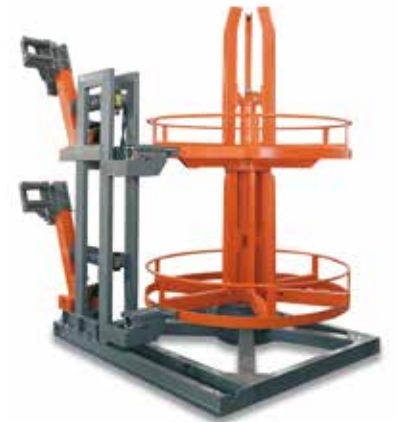
Double pay-off basement with pneumatic brake (2 coils 3T each) Double coil holder (3T)
