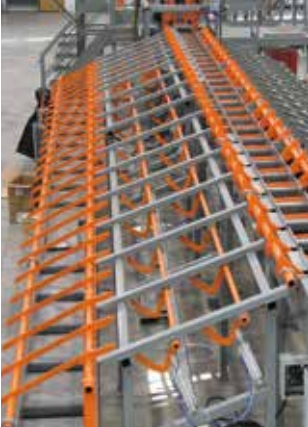
15. SDS: Pneumatic storage slide. Slide with 2 pneumatic arms for bars collection, able to transfer the bars to the close bending bench or bending robot.
