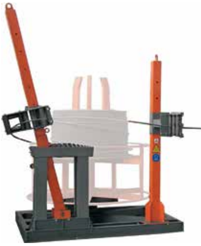
Base for pay-off with pneumatic brake with swinging arm (3,5 T)
