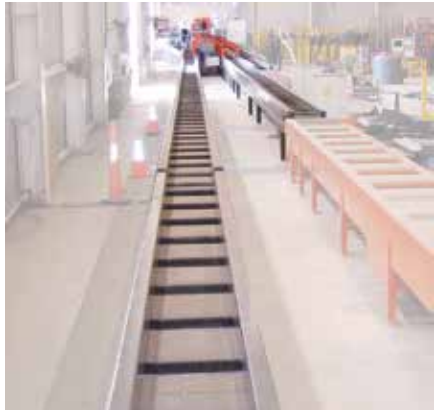
13. PT: Roller conveyor. Allows lengthwise transfer of bundles of bars.
