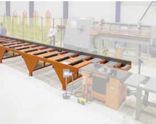
12 B12 MFC : Bending Bench with 2 roller tracks: 1 track with rubber-lined motorized rollers, and 1 roller track with idle rolls.
