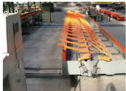
6. CPO: Mobile optimizing roller carriage. For storing and transferring bundles of bars cut to size towards subsequent machining operations.
