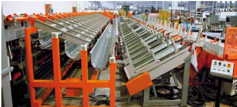
4. POCKET: Soundproofed cradle storage optimiser. it can be loaded and unloaded without any priority or sequence restriction.
