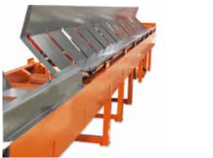
10. VRP: distribution tracks. They allow storing cut bars and act as storage unit for subsequent working operations.
